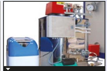
Steam generator capable to produce up to 50 kg/h.
